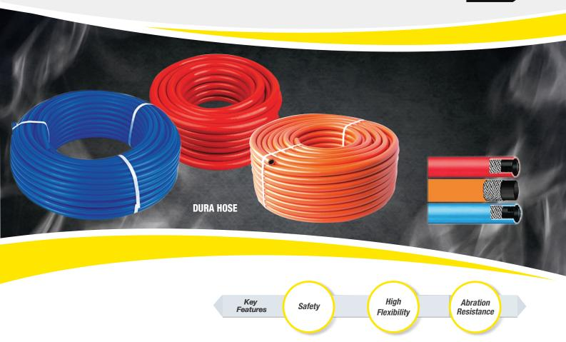
ESAB Dura Hoses are specially designed gas hoses for welding and oxy-fuel gas cutting with gas specific colour coding. The hoses are designed with a core of Black Synthetic Elastomer, High Tensile Polyester Yarn Reinforcement and Hyper Retardant Thermo-compound cover. The hoses are light weight, flexible with kink & crush resistance and very low bend radius. The Hoses conform to BIS standards.
